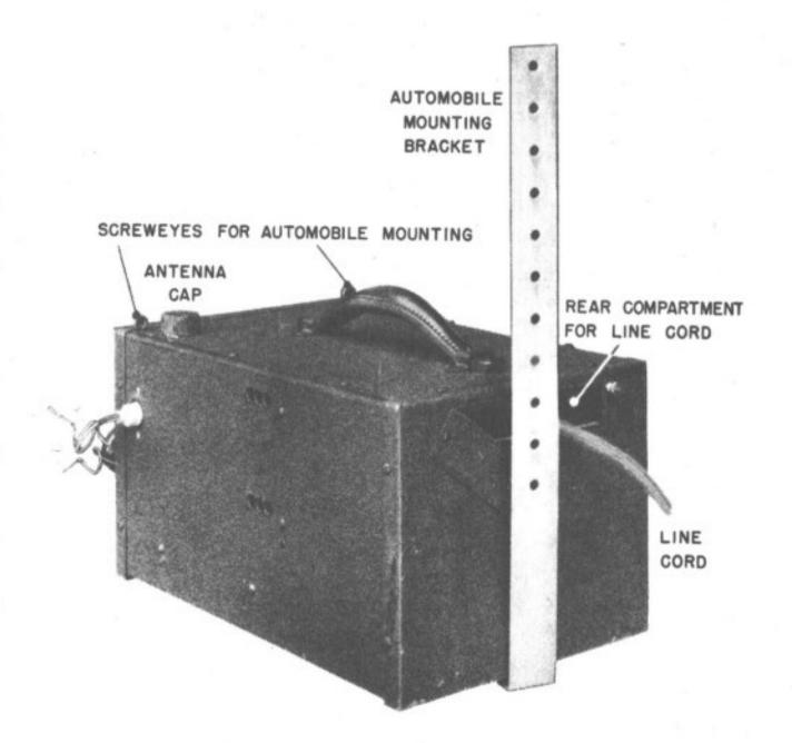
2 - MOUNTED IN AN AUTOMOBILE - For automobile mounting of the SKY TRAVELER - referring to the photographs - take the following steps:
